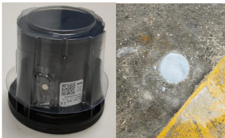
Figure 46: Photo sensor and its installation on the ground
